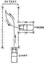
(The figure should be symmetrical, with the stakes placed to allow an over-all side clearance of approximately 18 inches at the finish. The entering lane should be wide enough to permit the movement if it is executed correctly.)
